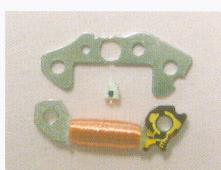
Stepping motor to convert electric signals into mechanical movements
